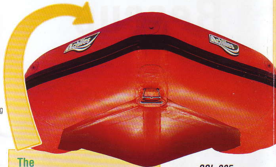
A nylon core is re-reinforced with Hypalon R outside and two layers of Neoprene inside.
